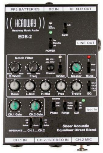
condenser microphone. No matter which configuration of inputs is used, the Channel 1 and Channel 2 inputs always get routed to individual gain controls for optimal mixing.
